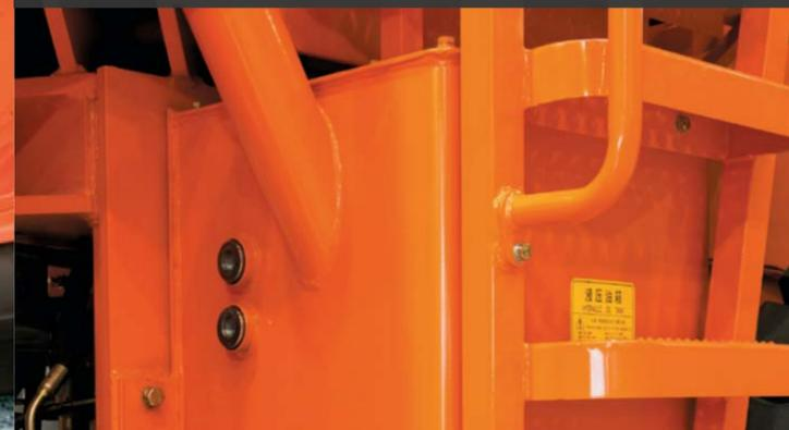
**Outdoor Power switch** Used to cut off battery power when necessary to enhance maintenance safety and convenience while protecting the battery and extending battery life when the device is parked for a long time. (SD300E, SD300, SD200)
